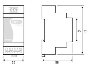
DIN rail housing; Width of 2 modules. Weight 80 g
