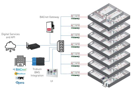
HELVAR IMAGINE is a complete lighting control and management solution. Built on top of open protocols such as DALI-2 and Ethernet, Imagine maximises on industry standards for easy installation and integration. It offers true scalability from a single room to entire buildings or campuses.
