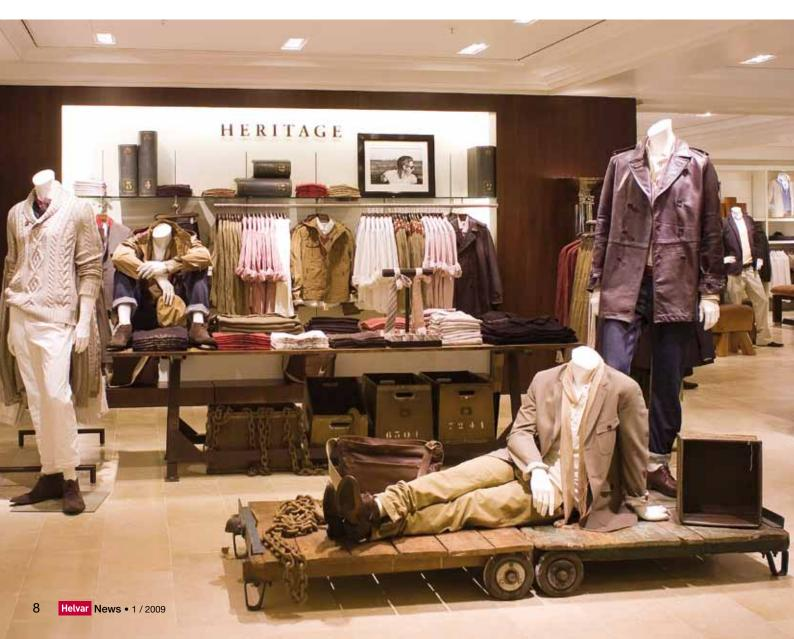
The finished Banana Republic lighting concept features a series of planar rafts with an array of angular adjustable flood and spot lights that have to work for the three different ceiling heights on each floor of the store: ranging from 2.3m to 4.8m.
